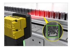
Electric vehicle DPM reading: Scan DPM codes on curved surface of cylindrical batteries
