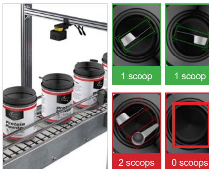
Assembly verification: Verify presence and quantity of serving scoops
