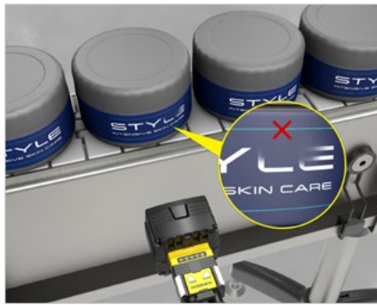
Defect detection: Inspect labels on final product packaging
